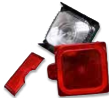
Rear and side lenses are individually replaceable.
